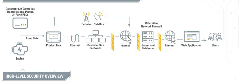
The technology for Cat Connect (Product Link TM Hardware) end-to-end system is designed with multi-layer security controls and safeguards to protect against unauthorized access and disclosure. High-level security safeguards include, but are not limited to:
