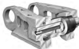
Sealed and Lubricated Track
