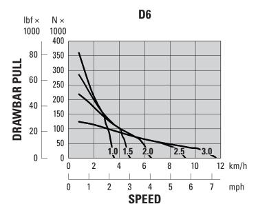
**NOTE:** Usable pull will depend on traction and weight of machine.
