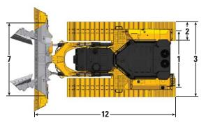
All dimensions above with Heavy Duty undercarriage with Moderate Service shoes of standard width
