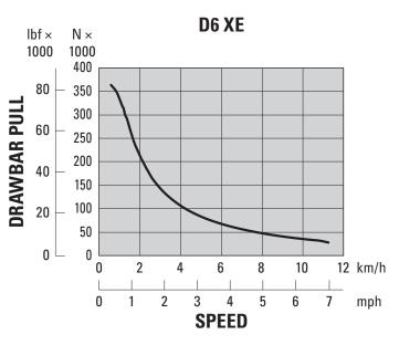
**NOTE:** Usable pull will depend on traction and weight of machine.
