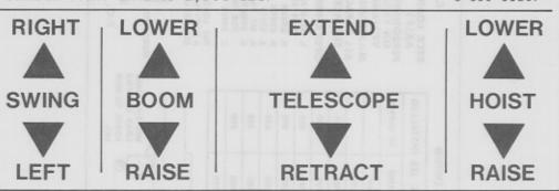
All controls are identified by placard and the directions of actuation for desired movement is indicated on the same placard.
