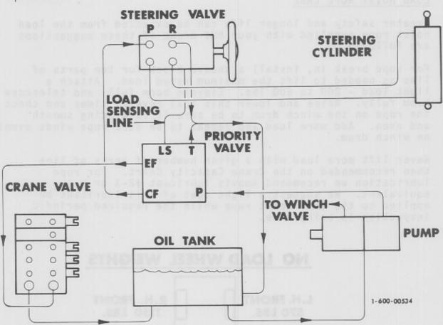
Oil from the small (rear) section of the pump goes into the Priority Valve at port "P". When no steering is required, the entire flow goes through the Priority Valve and leaves through port "EF" to the Crane Valve. The crane operating speed and power are not affected, since there is no loss of volume or pressure by passing through the Priority Valve.
