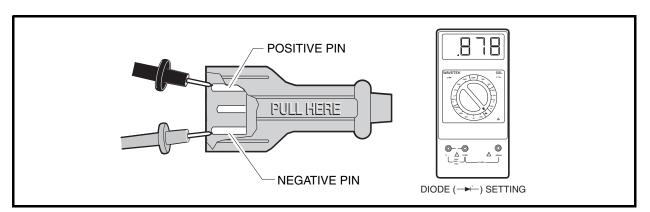
Figure 6-21 DC Plug Test - Probes Reversed
