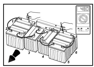
Figure 3-16 Battery Voltage Test – Style C Battery Configuration
