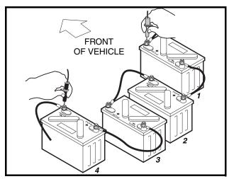
Figure 4-5 Battery Voltage Test – DS Villager 4
