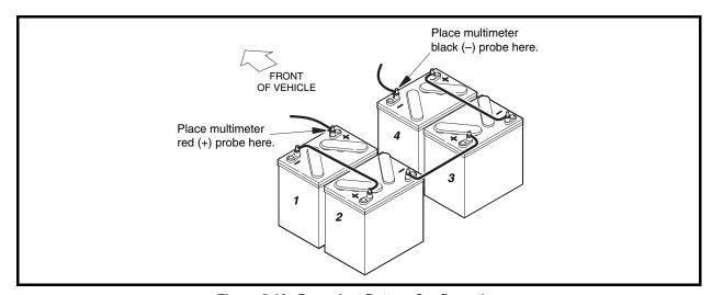
Figure 5-10 Precedent Battery Configuration
