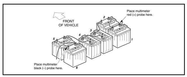
Figure 5-9 DS Battery Configuration
