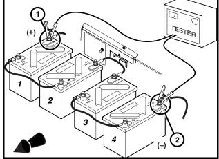
Figure 10-5 Battery Discharge Test – Precedent Style Figure 10-6 Battery Discharge Test – Precedent Style **A Battery Configuration**
