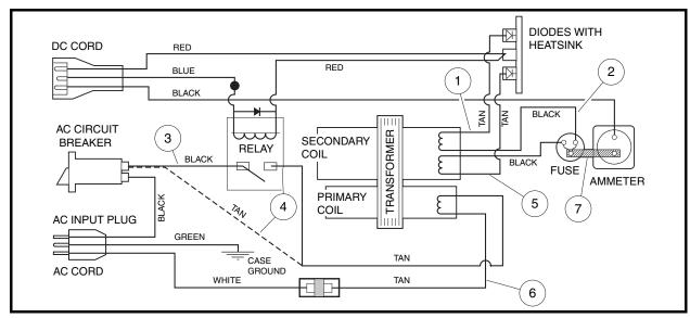
Figure 3-22 Transformer Test Wiring Diagram
