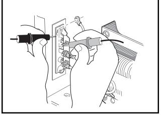
Figure 9-9 Diode Test
