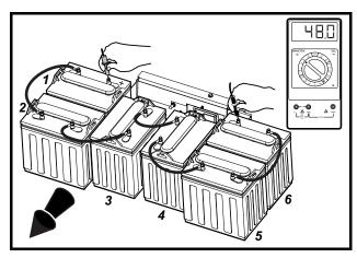
Figure 7-16 Battery Voltage Test – Precedent Style C Battery Configuration
