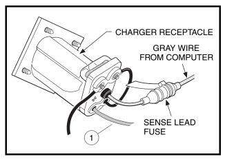
Figure 3-11 Receptacle Wire Connections (all vehicles except Precedent)
