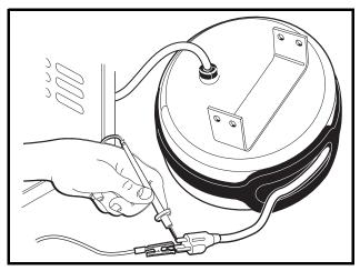
Figure 4-12 AC Circuit Continuity Test
