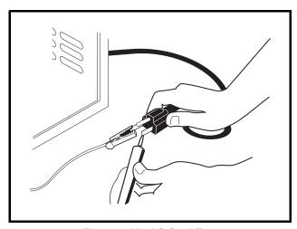
Figure 5-11 AC Cord Test
