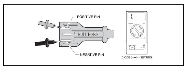
Figure 5-14 DC Plug Test
