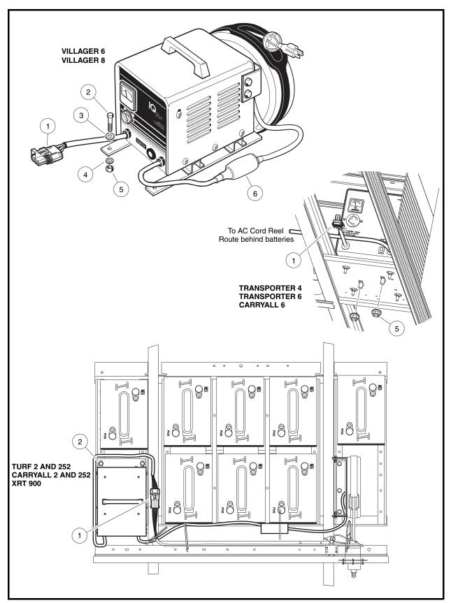
Figure 9-22 Onboard Charger Mounting Details
