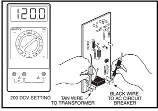
Figure 9-5 DC Circuit Test
