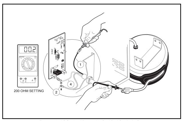
Figure 4-18 AC Cord and Retractable Cord Reel Continuity Test
