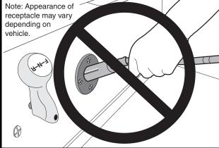
Figure 5-5 Incorrect DC Plug Removal
