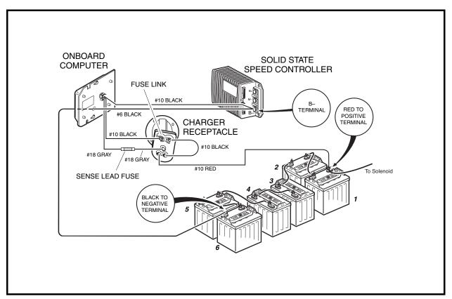
Figure 5-2 Charge Circuit and Battery Configuration – DS Vehicles
