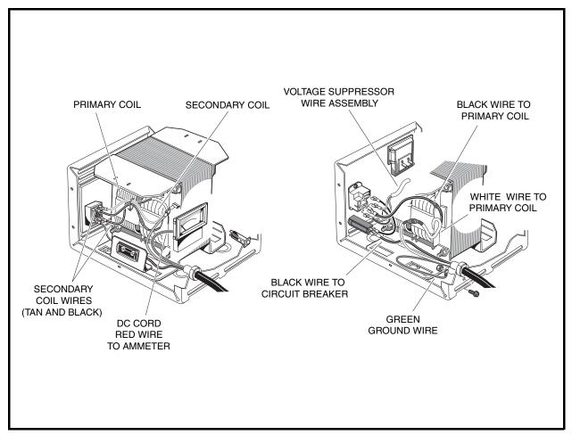
Figure 5-7 PowerDrive 2 Battery Charger
