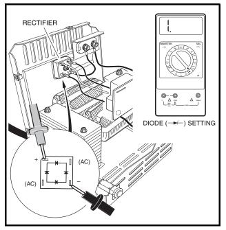
Figure 6-19 Rectifier Test – Probes Reversed
