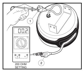
Figure 4-21 Retractable Cord Reel Test
