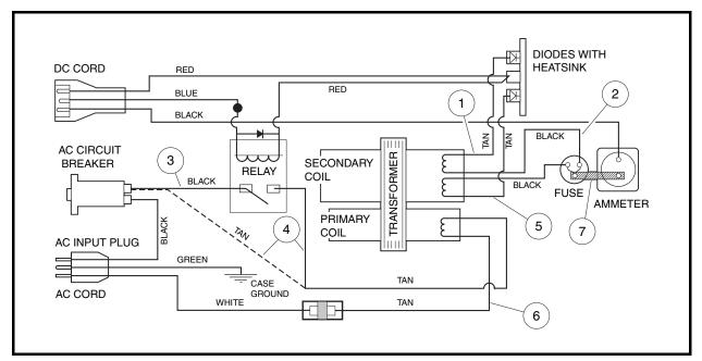
Figure 8-20 IQ Plus Charger Wiring Diagram (Relay Bypassed)
