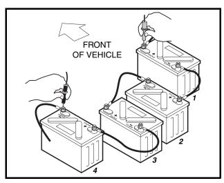
Figure 6-12 DS, DS Villager 4, 800, 810 and 850 Battery Configuration
