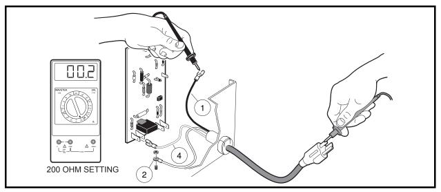
Figure 9-14 Short AC Cord Test
