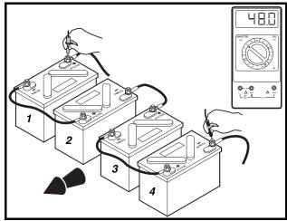
Figure 4-7 Battery Voltage Test – Precedent Style B
