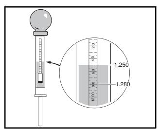
Figure 10-4 Hydrometer Test
