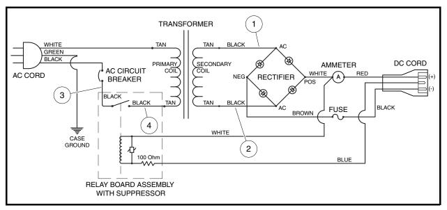
Figure 6-9 PowerDrive 3 Battery Charger Wiring Diagram (External Charger)
