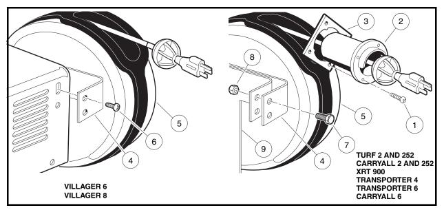
Figure 9-20 Retractable Cord Reel Mounting Details
