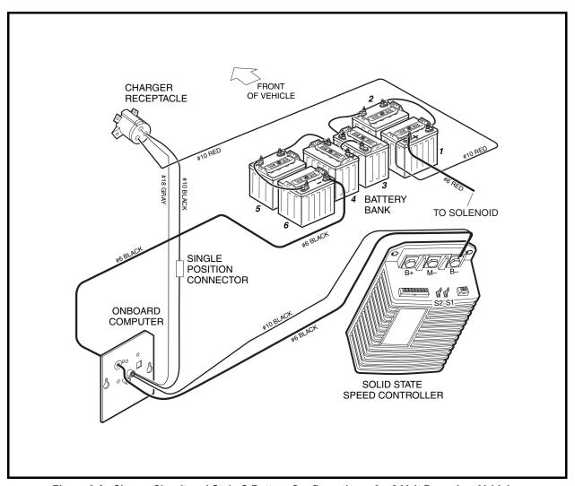
Figure 6-6 Charge Circuit and Style C Battery Configuration – 6 x 8-Volt Precedent Vehicles
