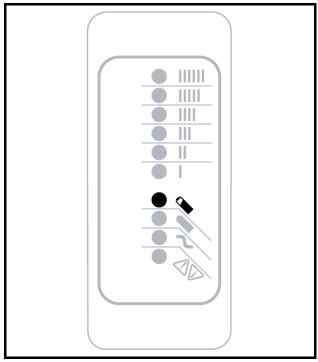
Figure 10-2 80% LED Flashes in Algorithm Display Mode
