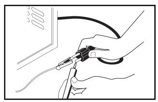
Figure 7-17 AC Cord Test
