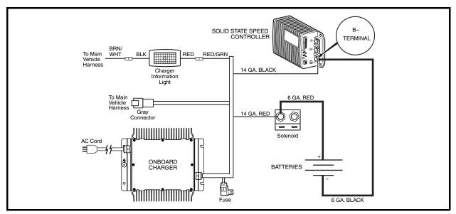
Figure 10-3 Charge Circuit
