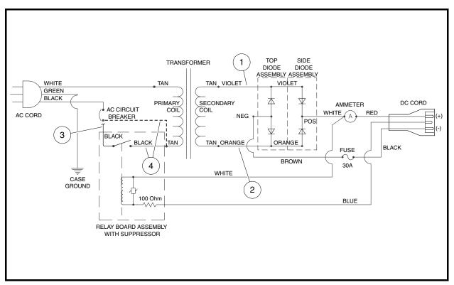
Figure 7-25 PowerDrive 3 Charger Wiring Diagram (Relay Bypassed)
