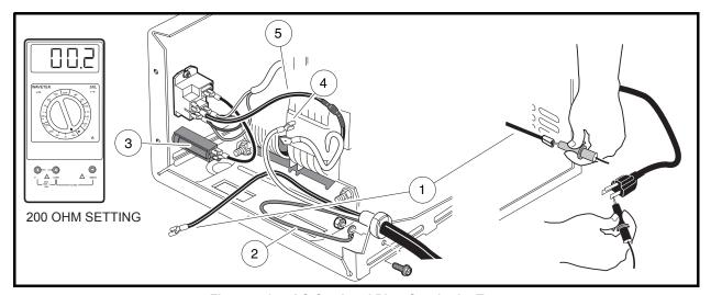
Figure 5-17 AC Cord and Plug Continuity Test
