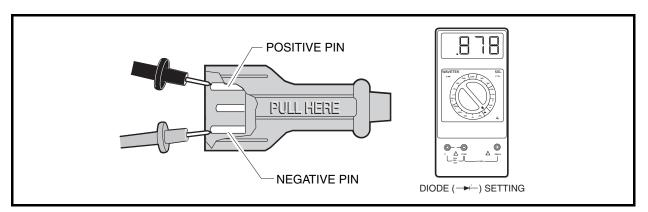
Figure 5-15 DC Plug Test - Probes Reversed
