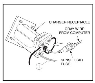
Figure 5-8 Receptacle Wire Connections (all vehicles except Precedent)
