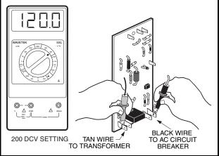
Figure 4-9 DC Circuit Test
