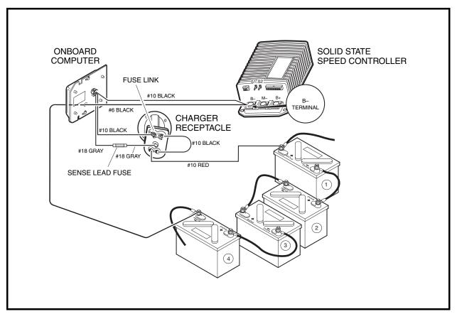
Figure 3-2 Charge Circuit and Battery Configuration - DS, DS Villager 4, 800, 810 and 850
