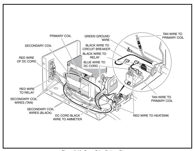
Figure 3-10 PowerDrive Battery Charger
