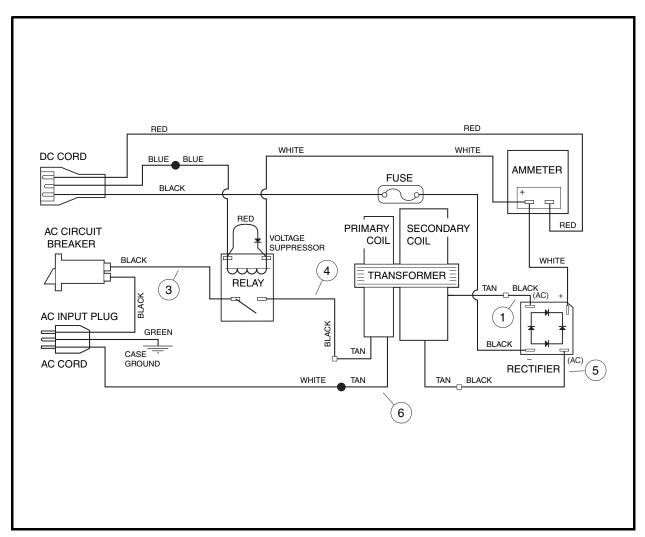
Figure 5-6 PowerDrive 2 Battery Charger Wiring Diagram (External Charger)
