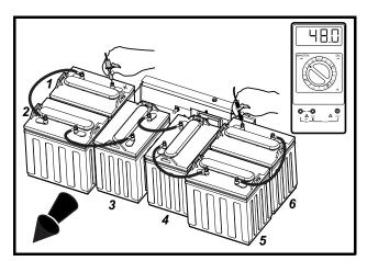
Figure 4-8 Battery Voltage Test – Precedent Style C
