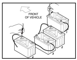
Figure 3-12 DS, DS Villager 4, 800, 810 and 850 Battery Voltage Test
