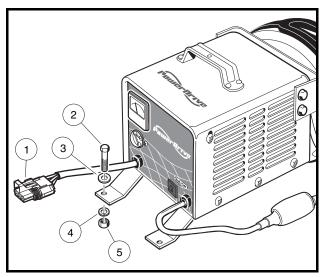
Figure 4-29 Onboard Charger Mounting – Precedent Vehicles
