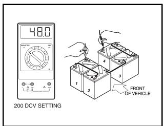
Figure 4-6 Battery Voltage Test – Precedent Style A
