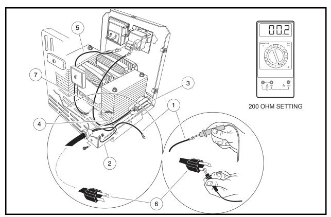
Figure 6-22 AC Cord and Plug Continuity Test
