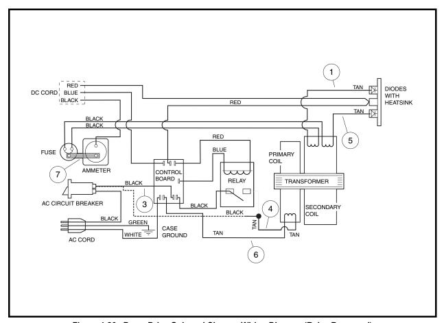
Figure 4-26 PowerDrive Onboard Charger Wiring Diagram (Relay Bypassed)
