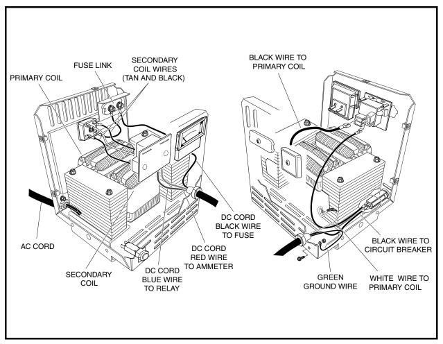
Figure 6-10 PowerDrive 3 Battery Charger Components - Model 26560
