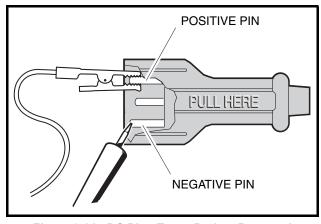
Figure 3-20 DC Plug Test
