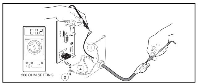
Figure 4-20 Short AC Cord Test
