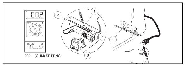
Figure 3-23 AC Cord and Plug Continuity Test
