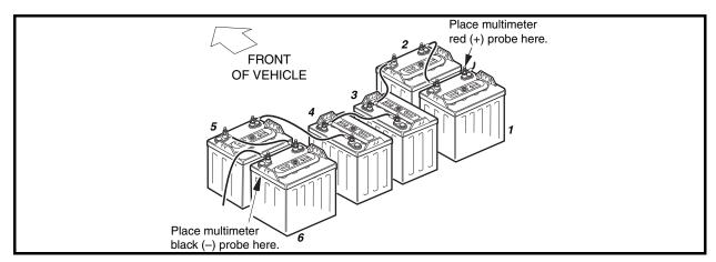
Figure 3-13 Turf 1 and Carryall 1 Battery Voltage Test
