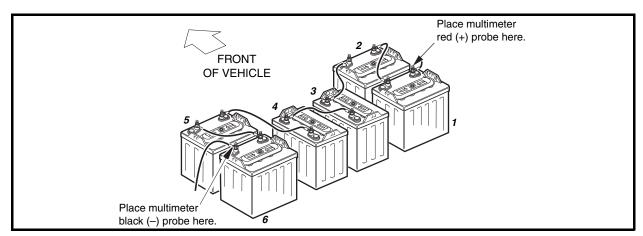
Figure 6-13 Turf 1 and Carryall 1 Battery Configuration
