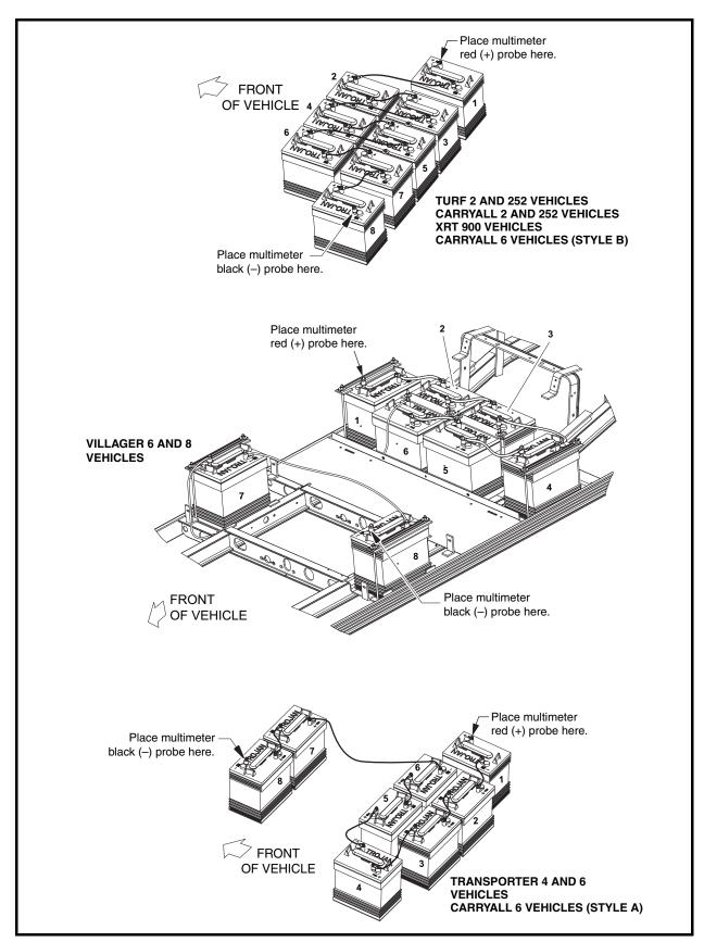
Figure 9-4 Battery Configurations
