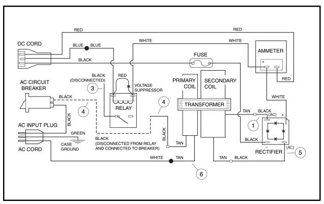
Figure 5-21 PowerDrive 2 Charger Wiring Diagram (Relay Bypassed)
