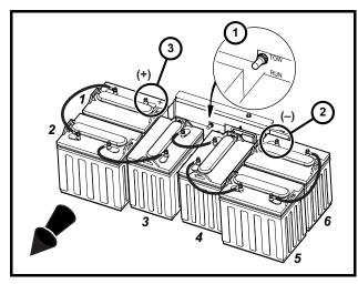
Figure 1-3 Precedent Battery Configuration – Style C
