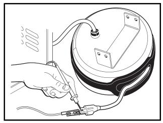
Figure 9-8 AC Circuit Continuity Test
