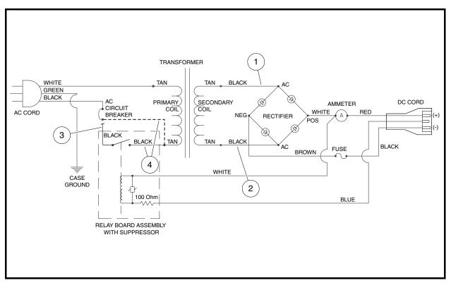
Figure 6-26 PowerDrive 3 Charger Wiring Diagram (Relay Bypassed)
