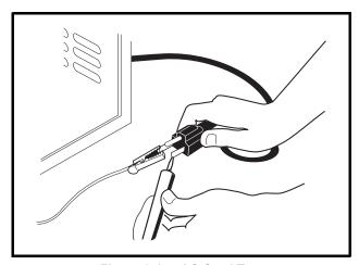
Figure 3-17 AC Cord Test
