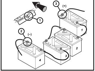
Figure 1-4 DS, DS Villager 4, 800, 810, 850 and Carryall 232 IQ System 4x12-volt Battery Configuration
