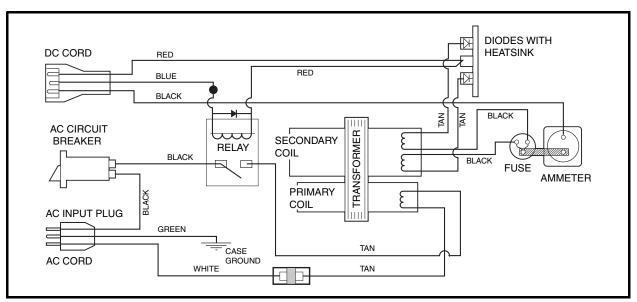
Figure 3-9 PowerDrive Battery Charger Wiring Diagram (External Charger)
