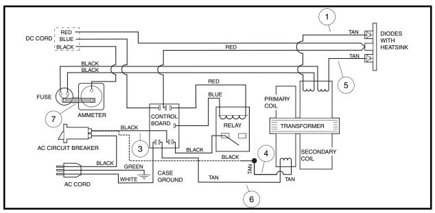
Figure 4-17 Transformer Test Wiring Diagram
