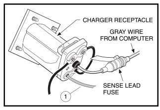
Figure 6-11 Receptacle Wire Connections (all vehicles except Precedent)
