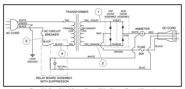
Figure 7-9 PowerDrive 3 Battery Charger Wiring Diagram (External Charger)
