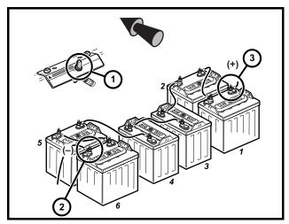
Figure 1-5 Turf1 and Carryall 1 Battery Configuration
