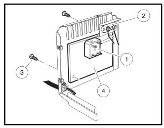
Figure 6-24 Rectifier/Heatsink Assembly
