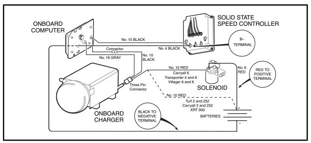
Figure 9-2 Charge Circuit
