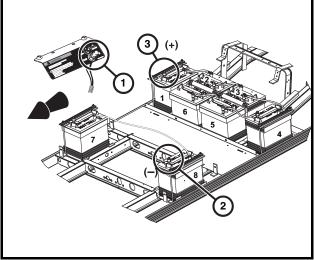
Figure 1-8 Villager 6 and 8 IQ Plus Battery Configuration
