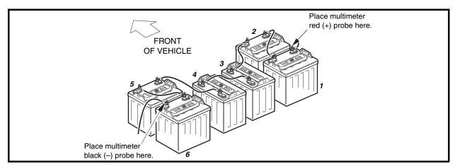
Figure 7-13 Turf 1 and Carryall 1 Battery Configuration
