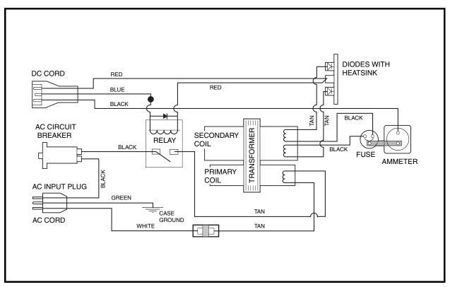
Figure 8-5 IQ Plus Battery Charger Wiring Diagram (External Charger)
