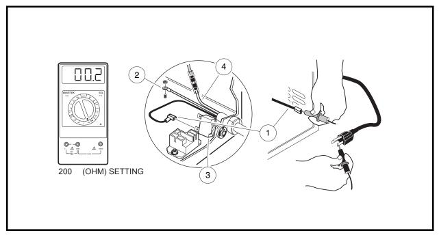
Figure 8-15 AC Cord and Plug Continuity Test
