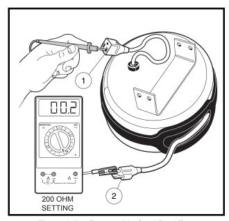
Figure 9-15 Retractable Cord Reel Test
