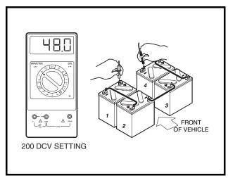
Figure 3-14 Battery Voltage Test – Style A Battery Configuration
