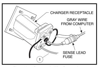
Figure 8-7 Receptacle Wire Connections
