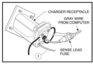
Figure 7-11 Receptacle Wire Connections (all vehicles except Precedent)
