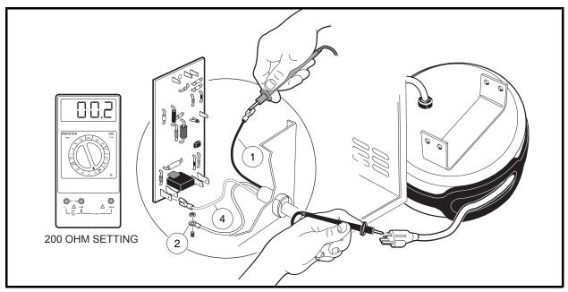
Figure 9-12 AC Cord and Retractable Cord Reel Continuity Test
