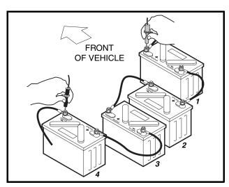
Figure 7-12 DS, DS Villager 4, 800, 810 and 850 Battery Configuration
