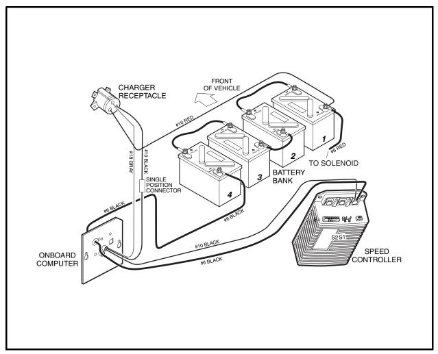
Figure 6-5 Charge Circuit and Style B Battery Configuration – 4 x 12-Volt Precedent Vehicles
