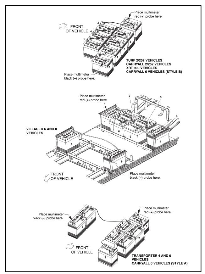
Figure 8-8 IQ Plus Battery Configuration
