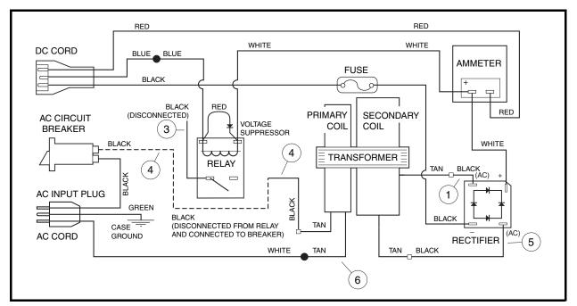
Figure 5-16 Transformer Test Wiring Diagram
