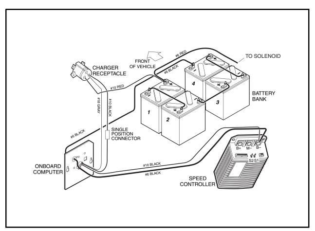
Figure 3-4 Charge Circuit and Style A Battery Configuration – 4 x 12-Volt Precedent Vehicles
