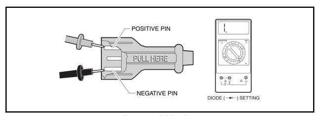
Figure 6-20 DC Plug Test
