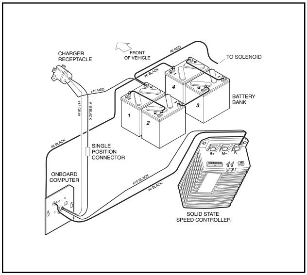
Figure 5-3 Charge Circuit and Battery Configuration - Precedent Vehicles
