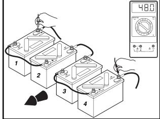
Figure 7-14 Battery Voltage Test – Precedent Style A Battery Configuration
