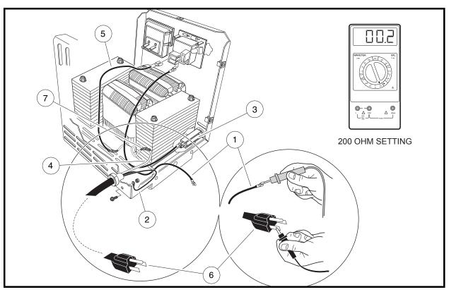
Figure 7-22 AC Cord and Plug Continuity Test
