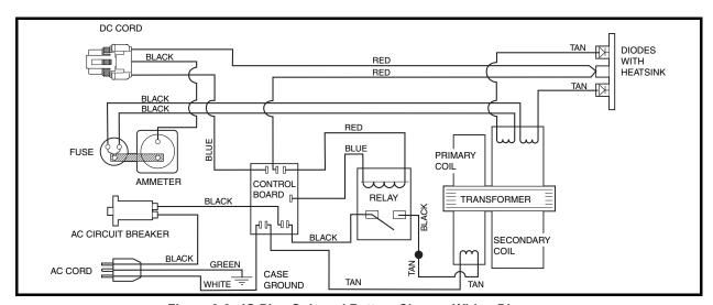
Figure 9-3 IQ Plus Onboard Battery Charger Wiring Diagram
