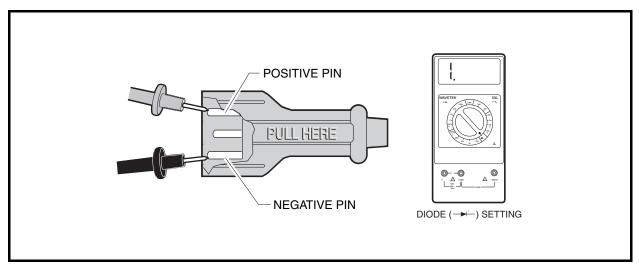
Figure 7-20 DC Plug Test
