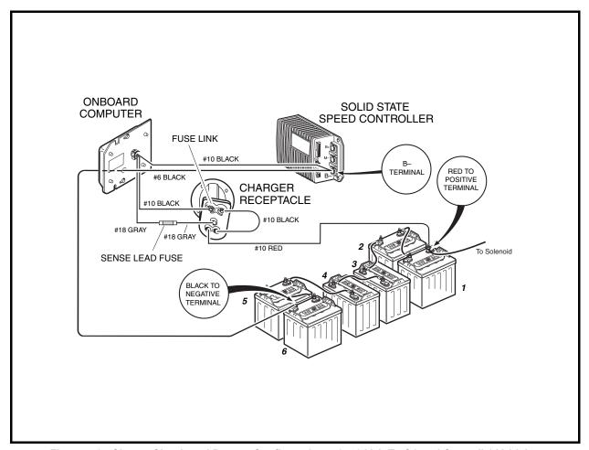
Figure 7-3 Charge Circuit and Battery Configuration – 6 x 8-Volt Turf 1 and Carryall 1 Vehicles
