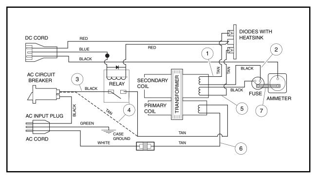
Figure 3-28 PowerDrive Charger Wiring Diagram (Relay Bypassed)
