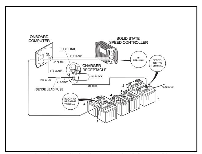
Figure 3-3 Charge Circuit and Battery Configuration – Turf 1 and Carryall 1
