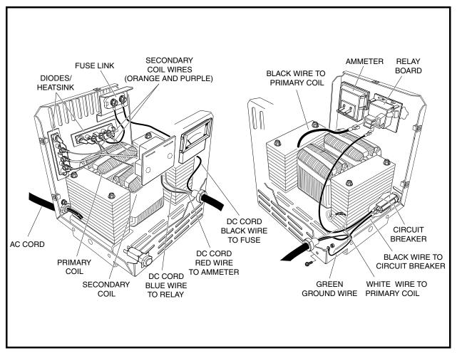
Figure 7-10 PowerDrive 3 Battery Charger Components - Model 26580
