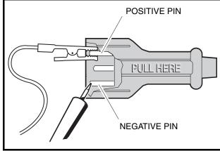
Figure 8-12 DC Plug Test
