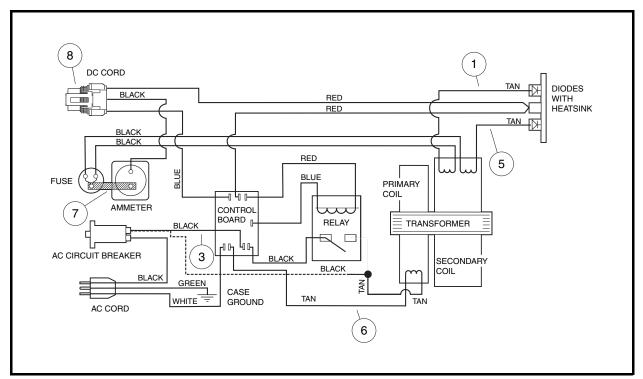
Figure 9-11 Transformer Test Wiring Diagram
