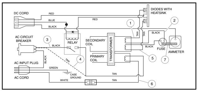
Figure 8-14 Transformer Test Wiring Diagram
