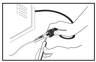
Figure 6-17 AC Cord Test
