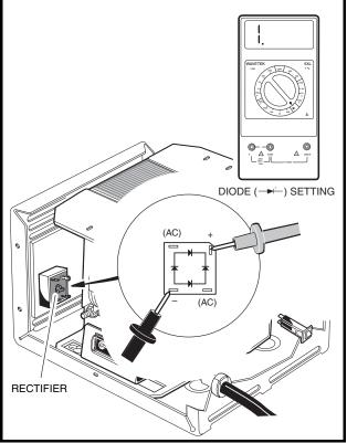
Figure 5-13 Rectifier Test – Probes Reversed
