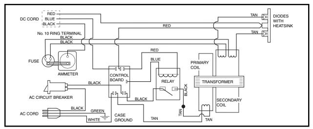
Figure 4-4 PowerDrive Onboard Battery Charger Wiring Diagram
