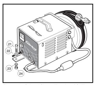
Figure 4-27 Onboard Charger Mounting – DS Villager
