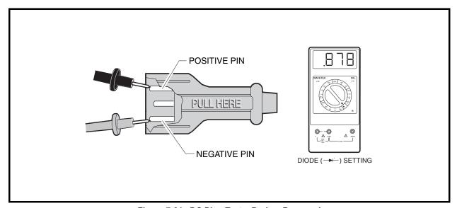
Figure 7-21 DC Plug Test – Probes Reversed
