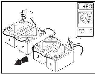
Figure 3-15 Battery Voltage Test – Style B Battery Configuration
