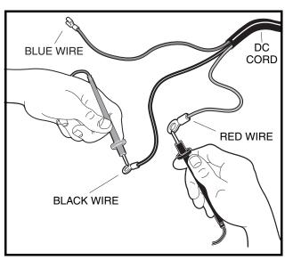
Figure 4-16 DC Cord Test (Probes Reversed) – DS Villager 4 Vehicles
