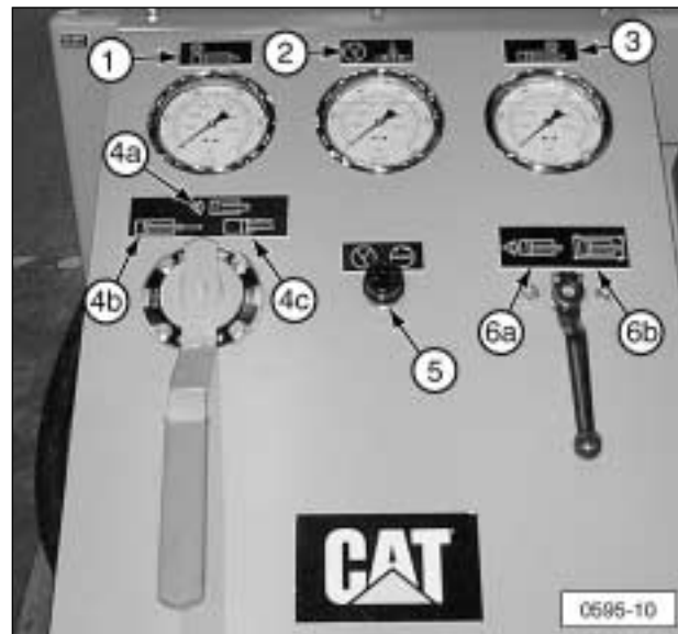
Illustration 2. (1) Cap Pressure. (2) Test Pressure. (3) Rod Pressure. (4a) Observe Cylinder. (4b) Rod Extend. (4c) Rod Retract. (5) Adjust Test Pressure. (6a) Observe Cylinder. (6b) Cylinder Cycle.
