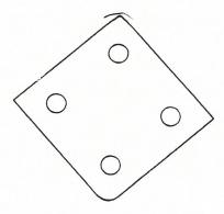
For regular cutting up to 3/8" angle iron, use this cutting edge of the blade which has a .50 radius
