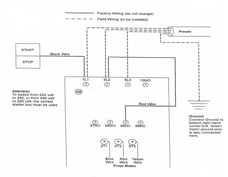
The only connections that you need to make are to the top terminals - 1L1, 3L2, 5L3 and to the groud. All other connections have been made and have been tested at the factory. If your machine runs in reverse, change 3L2 and 5L3.
