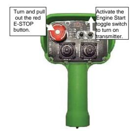
Push and hold the trigger on the inside of the remote handle to use the joystick crane controls.
