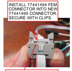
AFTER INSTALLING NEW CONNECTION, CUT OFF ORIGINAL CONNECTION AT END OF CABLE.
