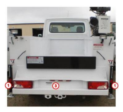
Place four red reflector decals, 70039057, item #1, at the sides and outer edges of the tailgate as shown.
