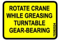
Crane worm gear bearing teeth must be lubricated weekly with extra heavy lubri-plate gear shield or equivalent. Cover all teeth with grease and leave no exposed metal surfaces showing.
