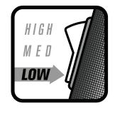
If there was no tendency for the drive wheels to lose traction and you desire greater slowing power, move the braking switch to the next highest position.
