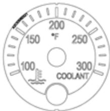
The water temperature gauge shows the temperature of the engine coolant. Under normal operating conditions the water temperature gauge should register between 165° and 205°F (74° and 90°C). Under certain conditions, somewhat higher temperatures may be acceptable. But the maximum allowable temperature is 210°F (99°C) with the cooling system pressurized, except for certain special engines. Check your engine manual to be sure.
