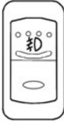
If your vehicle has fog lights, turn them ON or OFF with the control panel switch with the symbol shown above.
