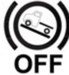
The hill hold feature is available as an option with certain automated transmissions. This feature holds the vehicle while on a hill to allow the operator to release the service brakes and press the accelerator. This feature will hold the vehicle if the vehicle is attempting to go up a hill from a stop in either drive or reverse.
