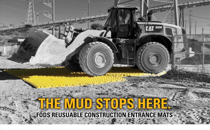
Do you have issues with vehicle tracking and sediment leaving your construction site? The FODS Construction Trackout Control Mats helps eliminate the tracking of mud and sediments outside of jobsites and is designed to be used on a construction entrance or exit that minimizes crossover contamination. FODS can be installed in under 30 minutes without heavy equipment.
