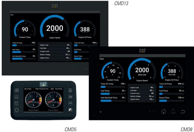
The CMD is available with a 5", 8" or 13" screen size. While CMD5 offers a more compact size and front and rear waterproof IP 66 rating, as well as appreciated tactile feel of the navigation keys.
